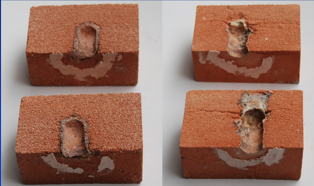
Results of vermiculite (left) and diatomite (right) insulating bricks corrosion test
